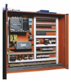
The CE conform electric installation is placed in an electric cabinet integrated at the rear side of the spindlestock.
