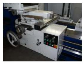
The compound slide consists of the carriage and the cross slide.
