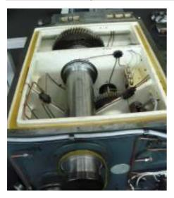
The triple bearing arrangement (two taper roller bearings and one cylindrical roller bearing) gives precise spindle properties with low radial run-outs.
