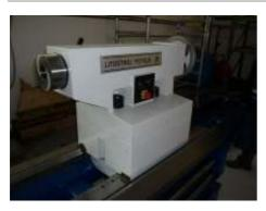
The rigid tailstock can be moved by means of an electric drive on the bed. The operation of the sleeve is manual.
