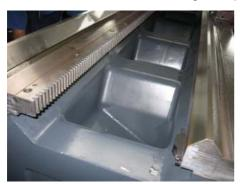
It is casted from grey iron with a homogeneous structure. The use of permanent sand cores improves vibration absorption properties. To avoid later distortion the bed undergoes natural and artificial aging.
